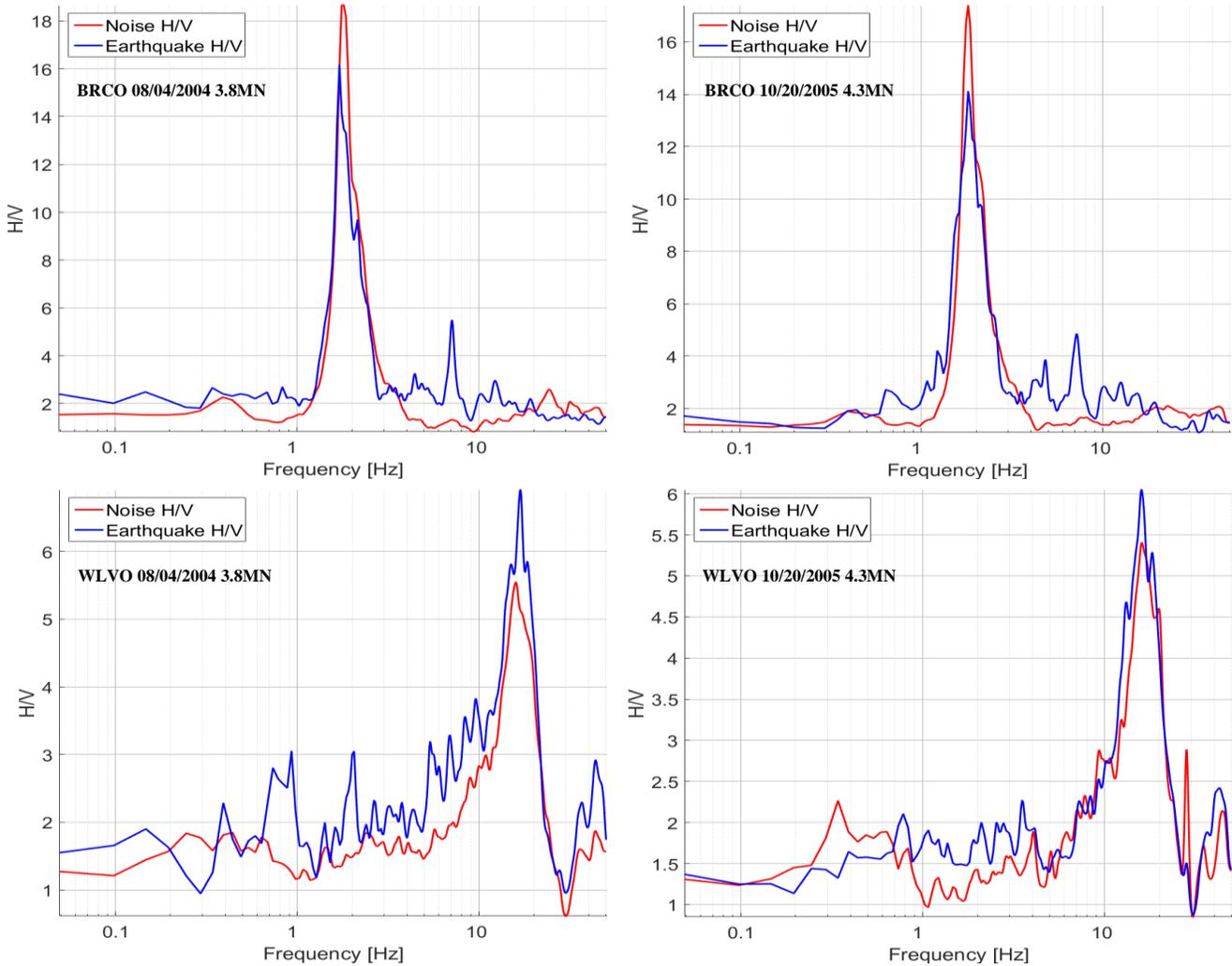
Figure 2: Comparison of HVSR from noise and earthquake data obtained for the two considered earthquakes (Table 2)
