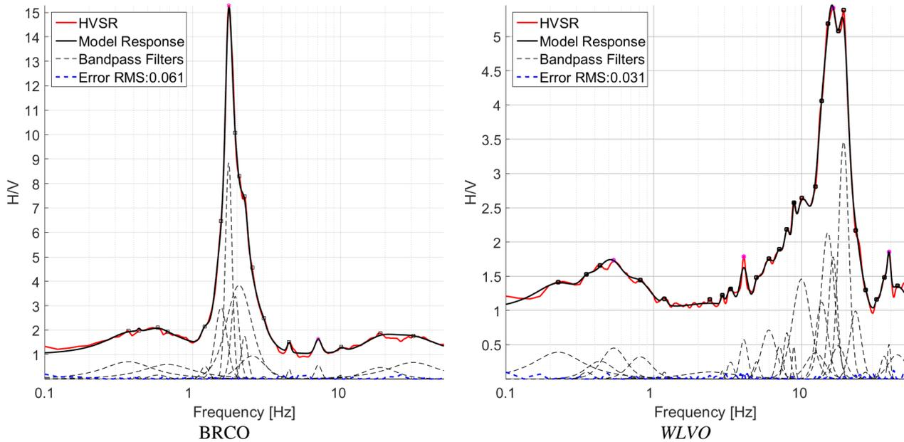
Figure 5: HVSr Models obtained from night time noise at the Bruce Peninsula (BRCO) and Wesleyville (WLVO) SOSN/Polaris stations. The points on the curves indicate the locations of the BPF center frequencies chosen for the approximation of the HVSr spectra
