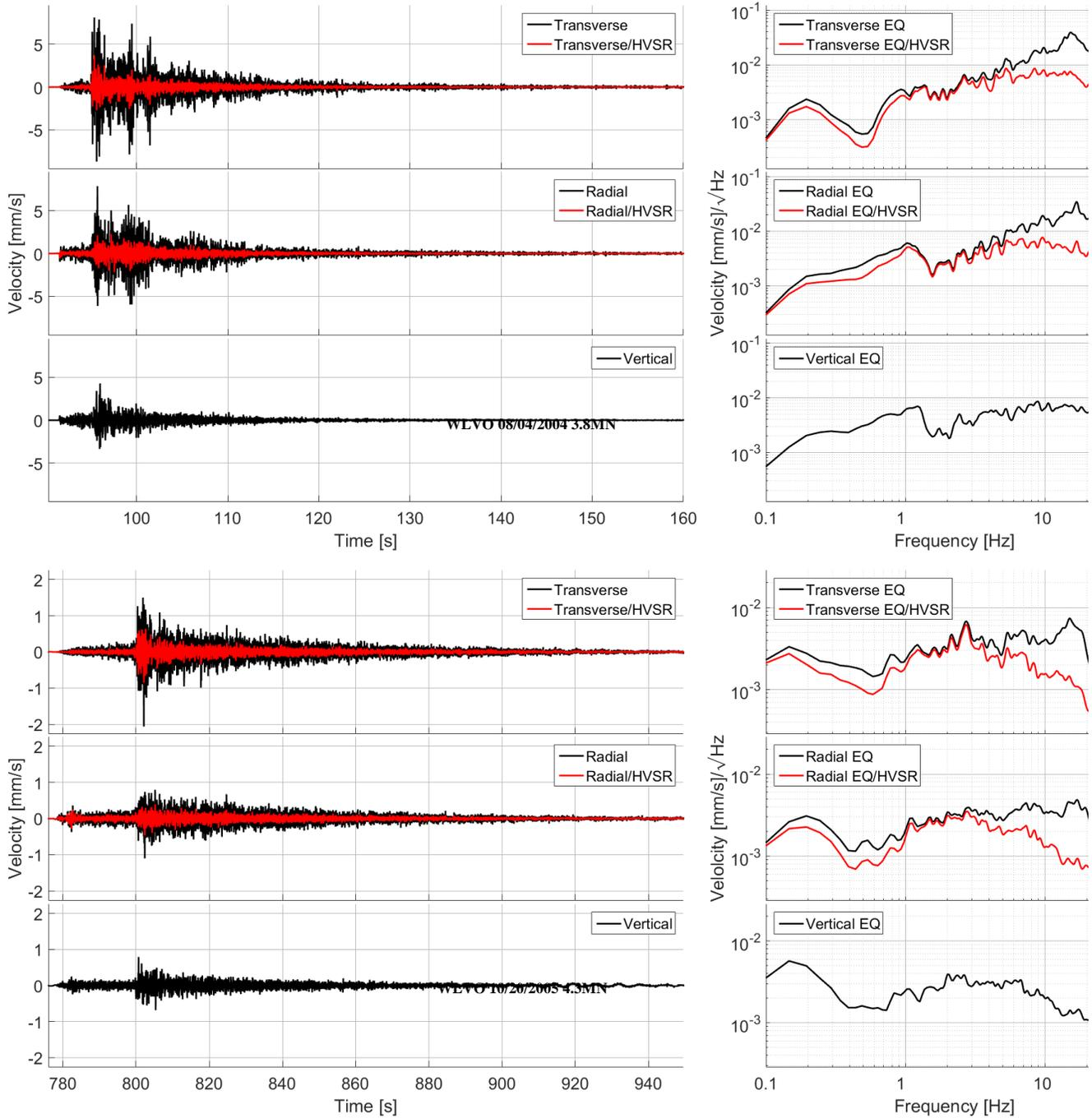
Figure 7: WLVO earthquake record (left) and spectra (right) for both considered earthquakes. (Black) original earthquake waveform and spectra, (Red) Waveforms and spectra of horizontal components corrected by HVSR model
