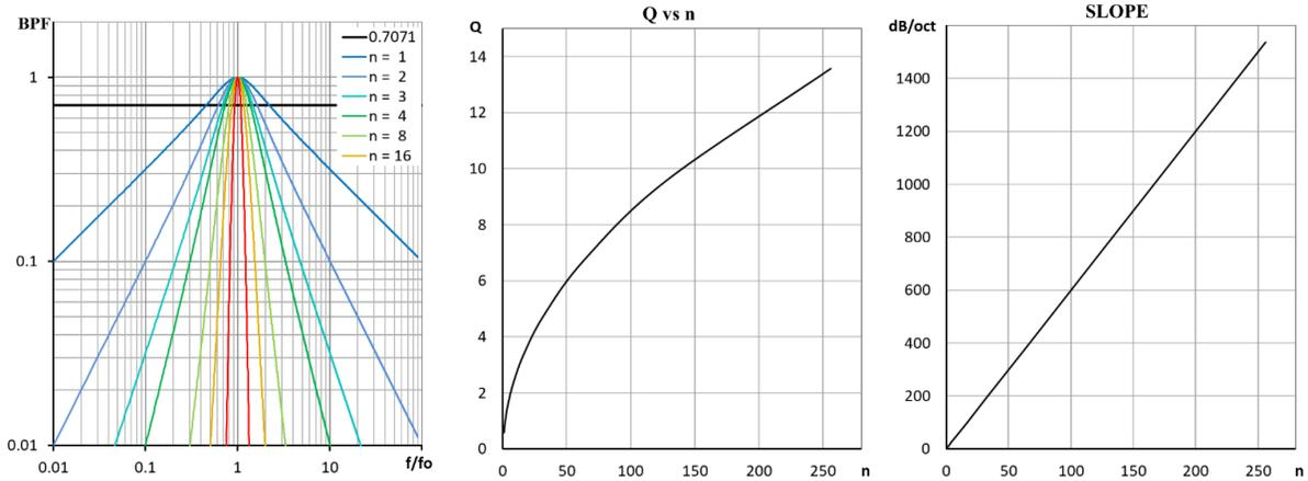
Figure 3: (left) Filter response for normalized  $f$ ; (middle and right) Quality factor and Slope as a function of slope steepness( $n$ ) Equations (4 and 6)
