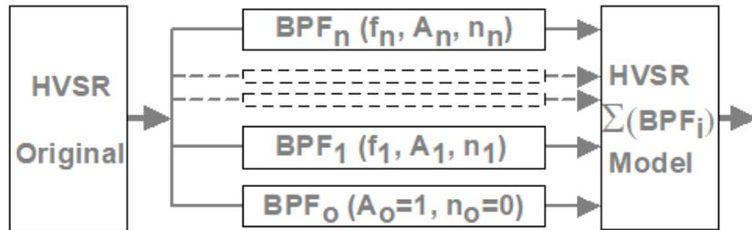
Figure 4: Simplified procedure for estimating a parametric HVSR spectral model
