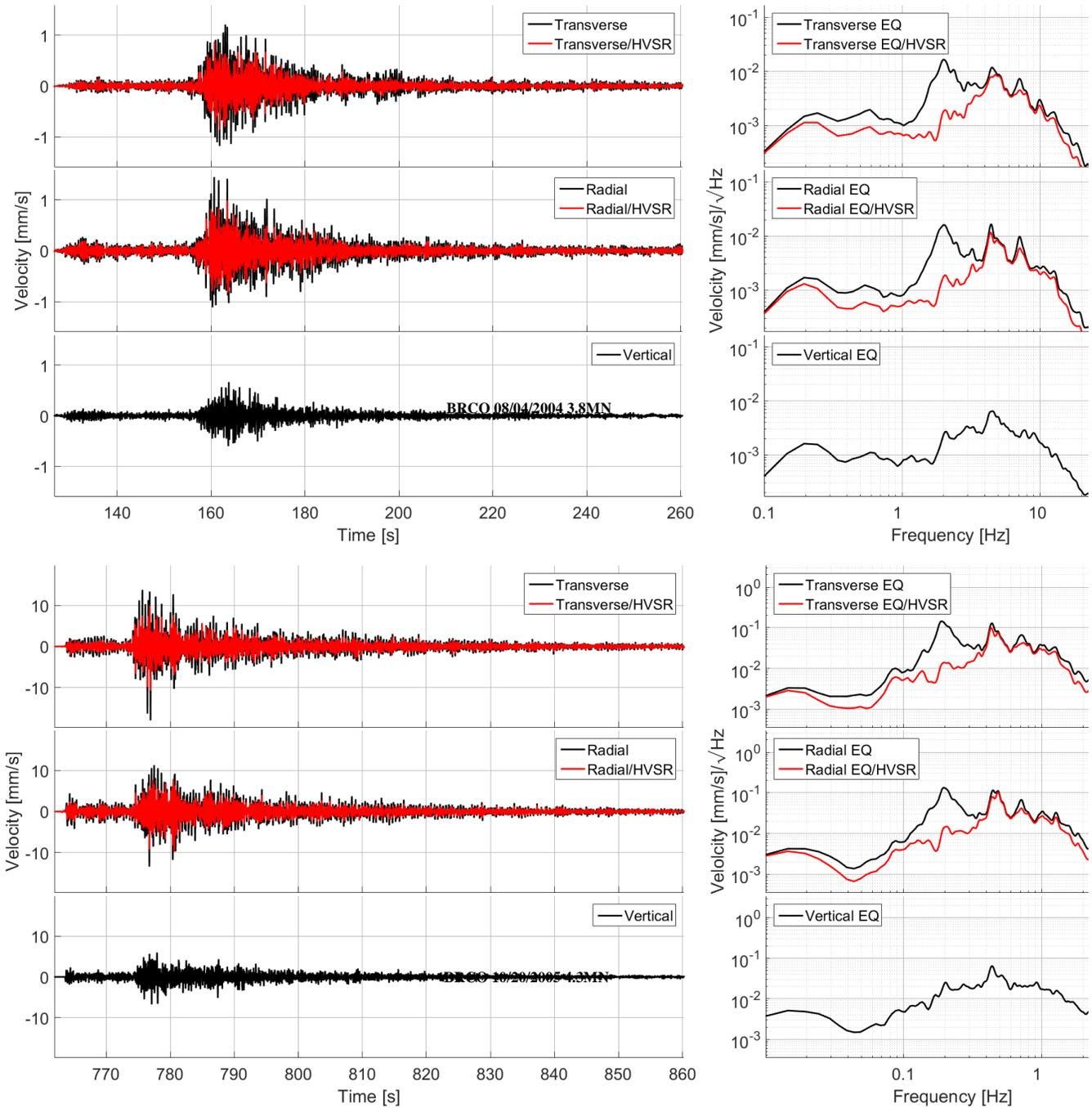
Figure 6: BRCO earthquake record (left) and spectra (right) for both considered earthquakes. (Black) original earthquake waveform and spectra, (Red) Waveforms and spectra of horizontal components corrected by HVSR model
